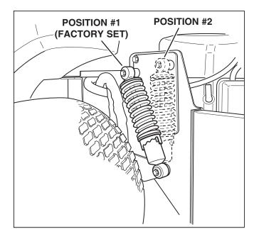
Figure 36. Rear Suspension Adjustments
